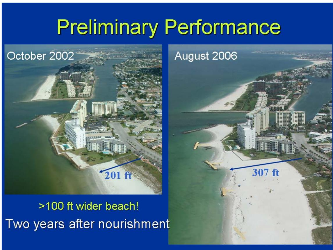
Due to the success of the experimental project in slowing erosion and saving money on renourishment, studies are underway to design permanent erosion control structures. The geotubes will be removed and replaced with rock structures as soon as possible given potential permitting constraints.
