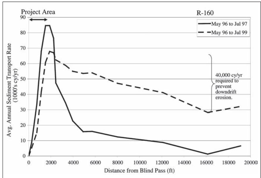
Figure 5. Short- and long-term net longshore sediment transport rate for Long Key following the 1996 nourishment project.
