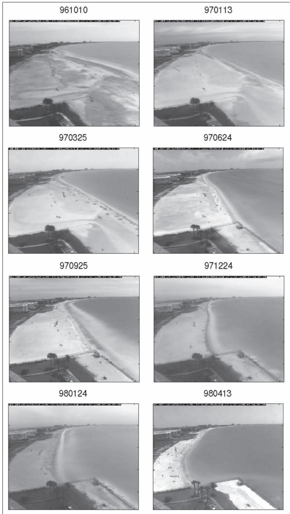
Figure 3. Video image time series showing the evolution of the 1996 nourishment over 18 months. The images are separated roughly by three-month intervals.
