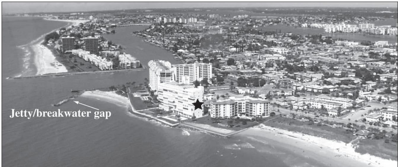
**Figure 2.** Oblique aerial photo looking north at Upham Beach and Blind Pass in October 2003, illustrates the typical condition of the project area prior to T-groin installation. Note the gap between the southern Blind Pass jetty and the detached breakwater. The condominium with the star housed the Argus video camera on its roof.
