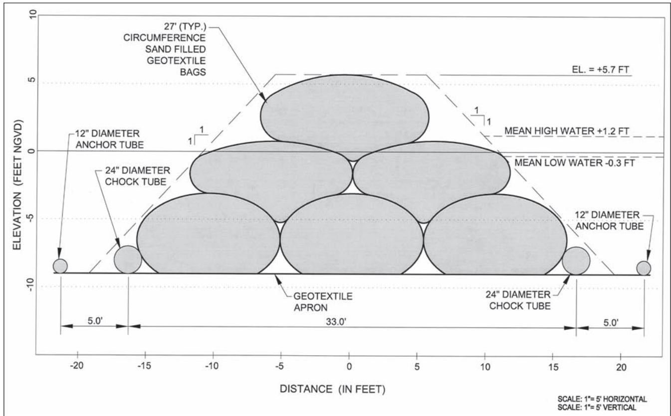
Figure 6. Cross-sectional view of the typical T-head illustrating the massive base of the structures, and the interlocking between geotextile layers.
