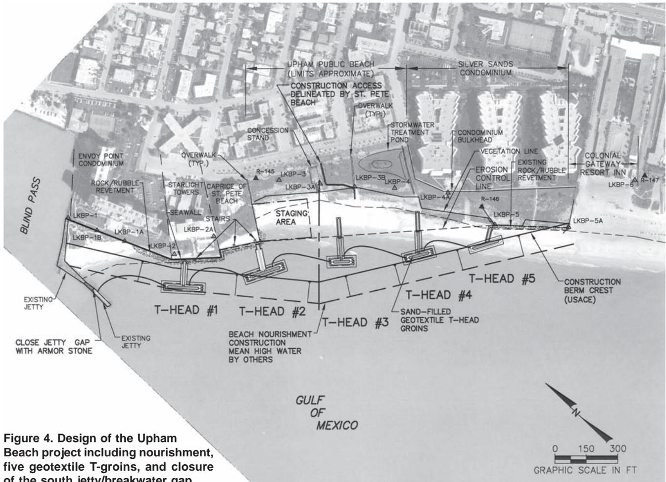
**Figure 4. Design of the Upham Beach project including nourishment, five geotextile T-groins, and closure of the south jetty/breakwater gap.**
