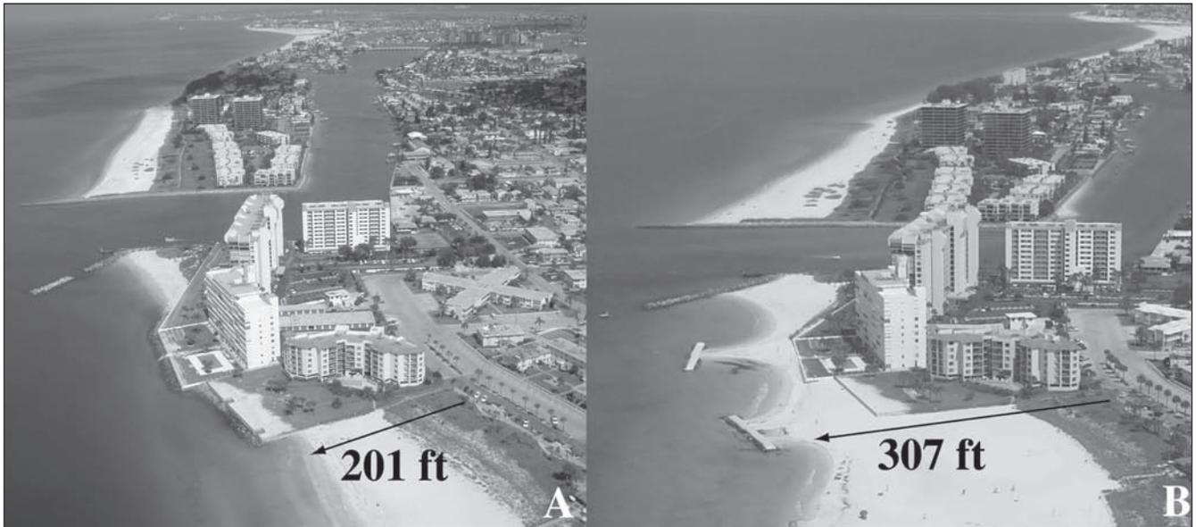
Figure 9. Aerial photos taken two years after the 2000 and 2004 nourishment projects in: A) October 2002 and B) August 2006. Survey data indicate that the beach is now over 100 ft wider than it was two years after the 2000 project.
