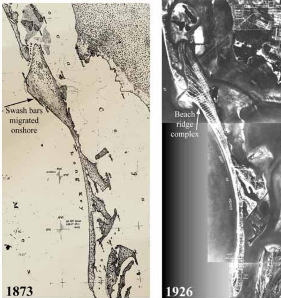
Long Key developed as a drumstick barrier island with a wide updrift end and a narrow downdrift end. Drumstick barriers develop when wave energy is refracted around the updrift ebb delta causing a local sediment transport reversal. On northern Long Key, sediment was transported onshore as swash bars that eventually welded to the beach. A prograding beach ridge complex formed on the updrift end of the island, creating the triangular shape (1873 above).
